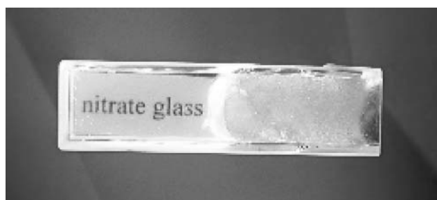
Fig. 2 Cuvette (20 mm long) filled with cadmium composite glass.
